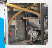
RUG 500-processes depolymerising plastic at 500°C, which has already been processed once, but without the excess CO2 that suffocates the Earth. Thanks to the low-energy decomposition of plastic, the opportunity to develop ecology is offered.
